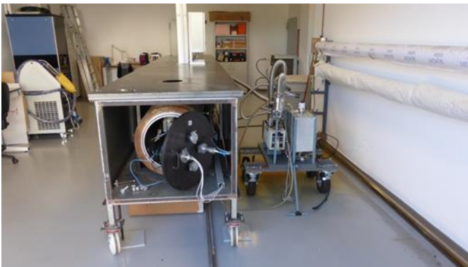
Figure 116. View of the HEATREC test chamber to measure heat losses in solar receiver tubes (left) and RESOL test bench to measure the receiver's optical efficiency (right).
