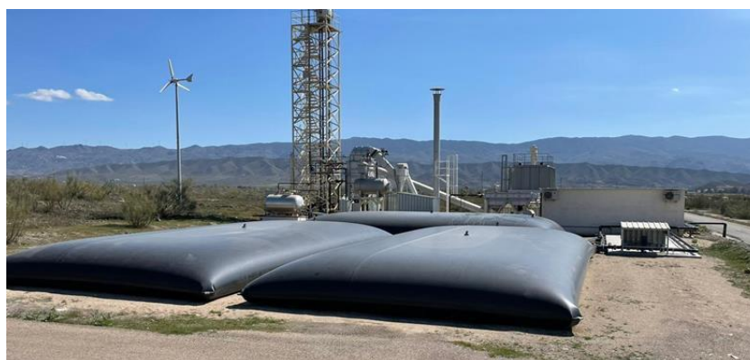
Figure 88. Containers filled with real seawater for desalination tests in closed loop.
