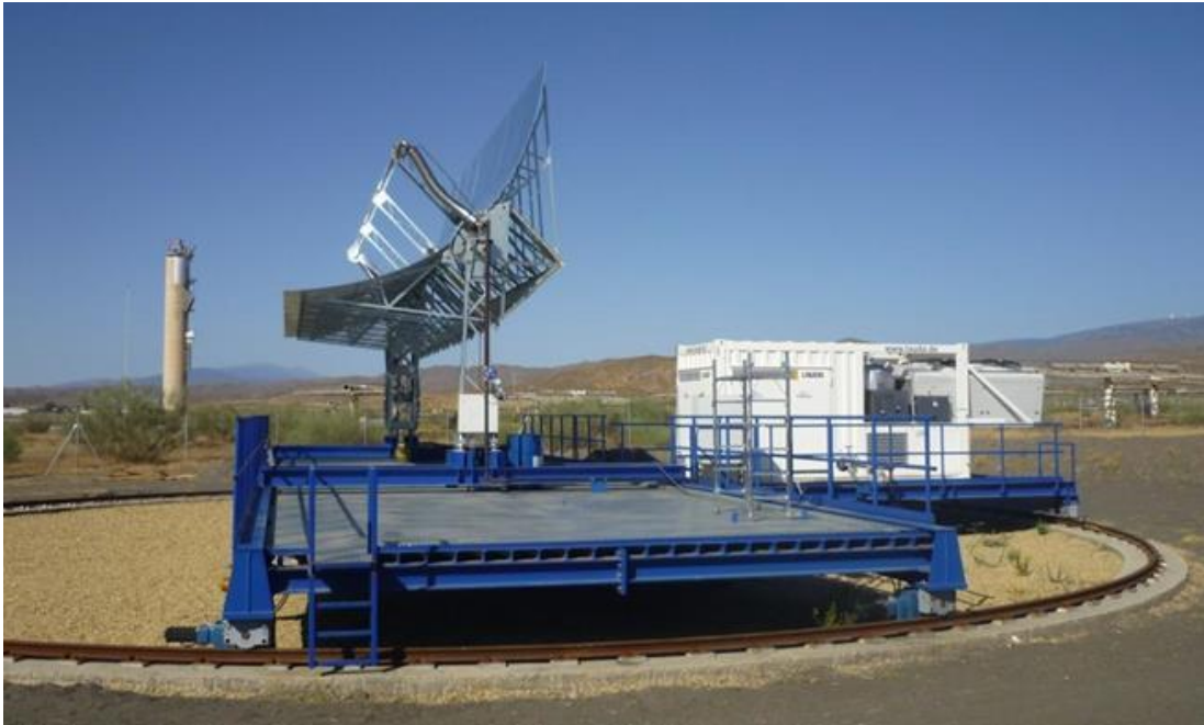
Figure 60. Side view of KONTAS test bench and the heating/cooling unit (right side).
