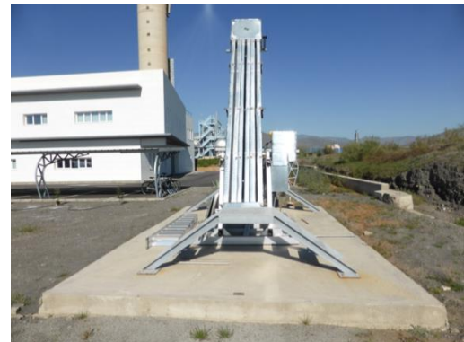
Figure 116. View of the HEATREC test chamber to measure heat losses in solar receiver tubes (left) and RESOL test bench to measure the receiver's optical efficiency (right).
