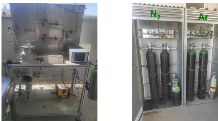
Figure 102. Left: Solar pilot plant for photocatalytic generation of hydrogen; Right: Gas ( N_2 and Ar) conduction systems.
