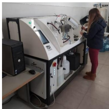
Figure 124. Bench-scale unit for testing MD with flat-sheet membranes.
