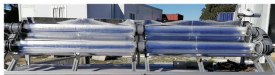
Figure 48. New CPC photoreactor designed in a collaborative action among the Solar Treatment of Water Research Unit at PSA (CIEMAT) with the University of Évora for testing small concentrations of photocatalysts to eliminate microcontaminants present in urban wastewaters.
