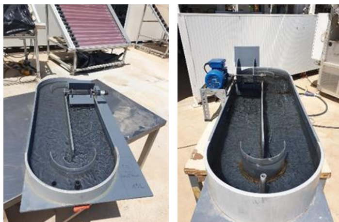
Figure 94. Raceway Pond Reactor with capacities of (left) 15 L and 5 cm of liquid depth and (right) 90 L and 15 cm of liquid depth.
