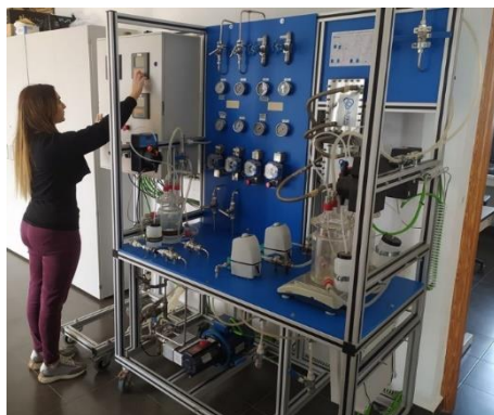
Figure 125. Bench-scale unit for testing FO and PRO.
