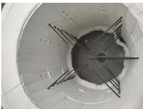
Figure 81. Picture taken from the top of the tank, showing its internal room and thermocouples at different lengths and radial positions.
