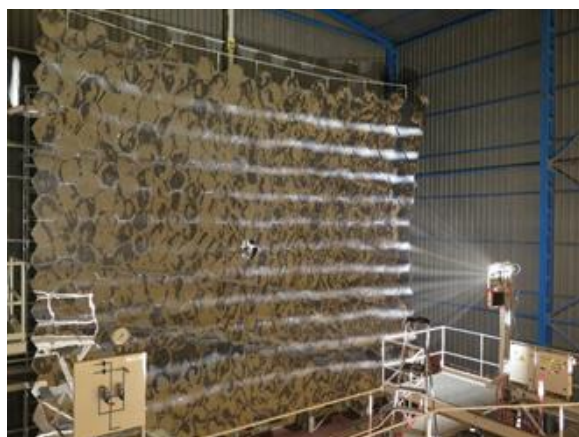
Figure 74. Interior view of the PSA SF-60 Solar Furnace in operation.
