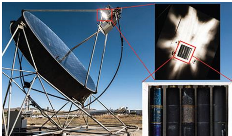
Figure 70. Accelerated aging tests of steel samples at a parabolic-dish DISTAL- II
