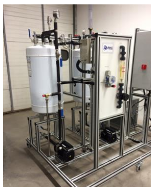
Figure 123. Bench-scale unit for testing membranes on isobaric MD.
