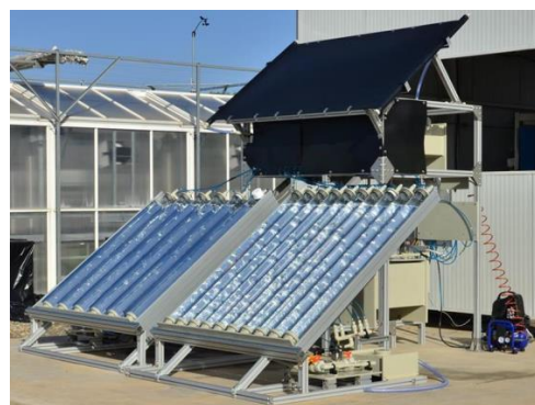
Figure 93. View of new CPC and U-type photoreactors (NOVO 75 V 1.0).
