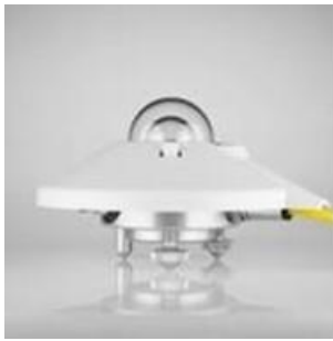
Figure 105. CUV-5 radiometer (left). View of all solar UV radiometers, horizontal (centre) and inclined (right) setup used in the Solar Treatment of Water Unit.
