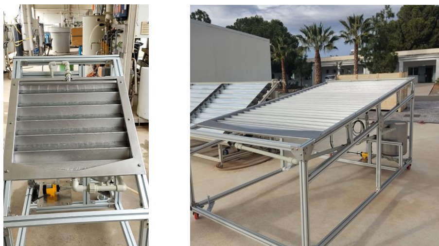
Figure 39. Multistep cascade reactors developed and tested in ENERGICA project for water treatment: (left) pilot plant of 5 L capacity and (right) pilot plant of 50 L containing TiO 2 immobilized in stainless steel stairs.
