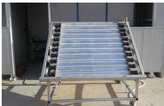
Figure 92. View of 2 m 2 -CPC coupled to Electro-Fenton pilot plant (ELECTROX).
