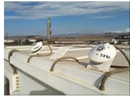
Figure 105. CUV-5 radiometer (left). View of all solar UV radiometers, horizontal (centre) and inclined (right) setup used in the Solar Treatment of Water Unit.
