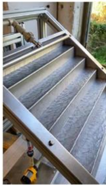
Figure 97. Solar waterfall reactor photography (left) and scheme (right).
