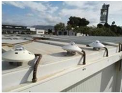
Figure 105. CUV-5 radiometer (left). View of all solar UV radiometers, horizontal (centre) and inclined (right) setup used in the Solar Treatment of Water Unit.
