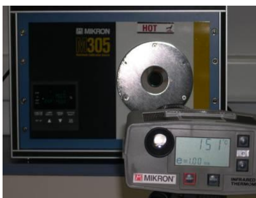
Figure 113. IR sensor calibration using a black body.
