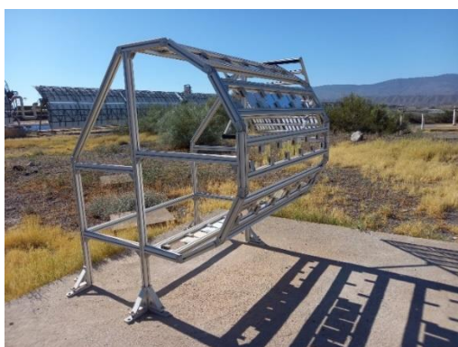
Figure 27. Left: Reflector samples exposed at different inclinations to achieved several soiling levels. Right: portable reflectometers included in the study of the transfer functions.
