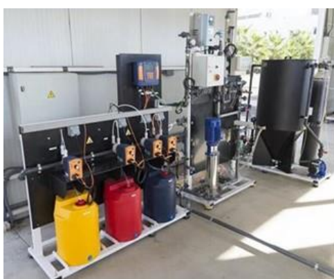
Figure 101. Left: Nanofiltration pilot plant. Right: New labview interface for control and automatic operation of the pilot plant.
