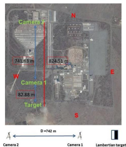
Figure 20. Extinction measurement system layout at PSA.
